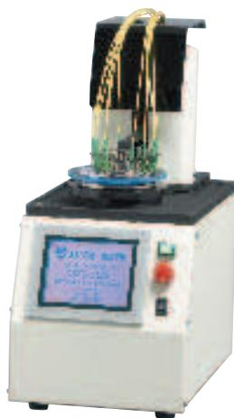
This model is another highest grade of our polishing machines with excellent capability of max. 24 axis simultaneous polishing, versatility for various connector such as MT ferrule. It features LCD touch panel for programing various connector polishing processes to achieve easier operation. Additionally, it features active polishing pressure control with load-cell sensor and stepping motor to achieve excellent polishing result.
