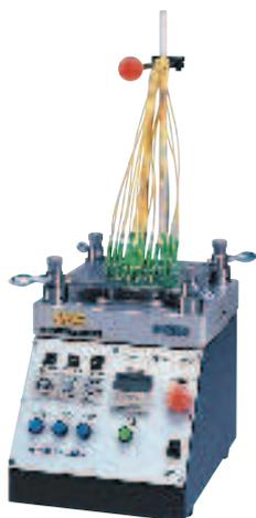
Succeeding higher 550S' essential mass-production adaptability and versatility, this features 4 timers instead of touch panel on the front panel to maintain operational certainty based on eye-checking to reduce operator's mistake. It also features speed adjuster of turntable and voltage - free power input.
